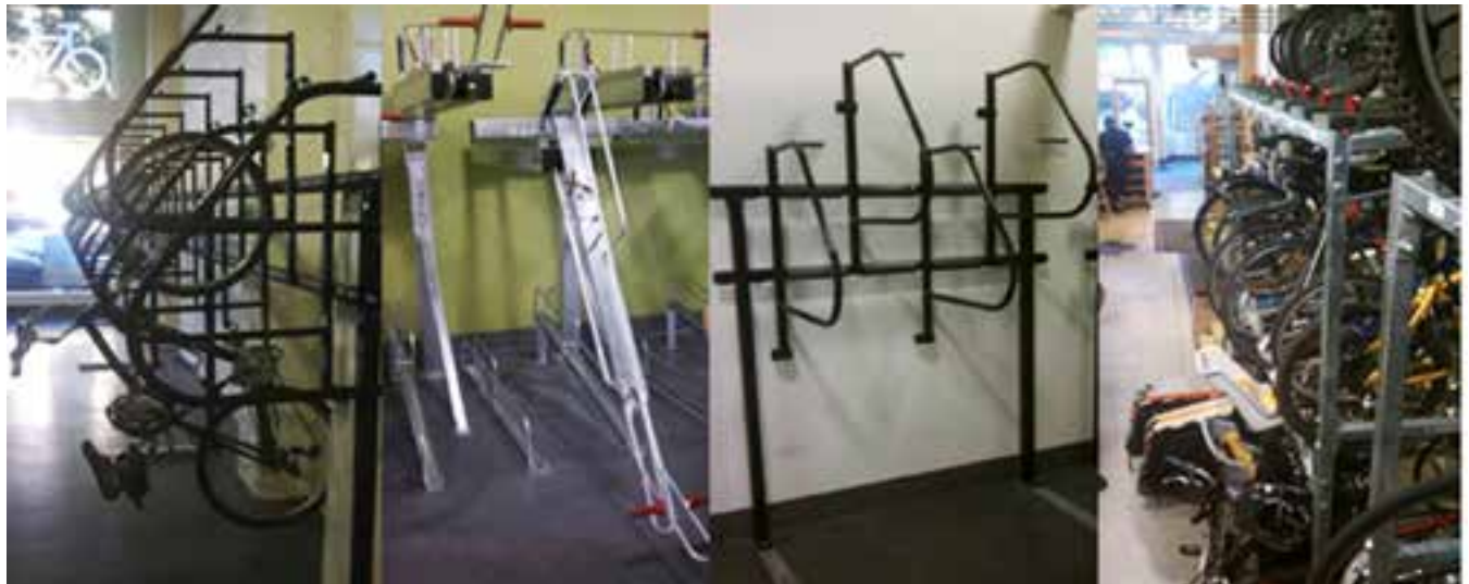
Figure 8 Example Indoor Racks (from left to right): Wall, Stacked, Wall, and Stacked
