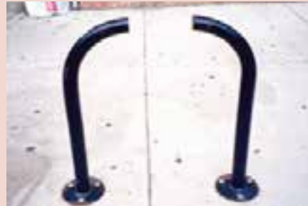
Round tubes cut with pipe cutter and rust under powder coat finish*
