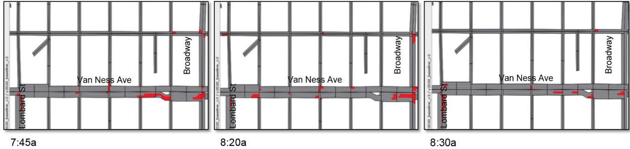
FIGURE 15. SAMPLE QUEUE LENGTH COMPARISON BETWEEN SCENARIOS WITH A SINGLE AND DOUBLE LEFT TURN LANE ON SOUTHBOUND VAN NESS AT BROADWAY
