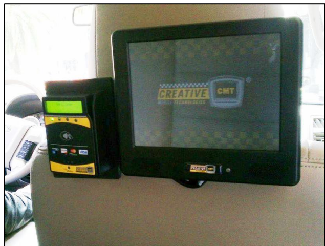
Passenger information monitor (PIM) & back seat credit card swipe used by Creative Mobile Technology (CMT)
