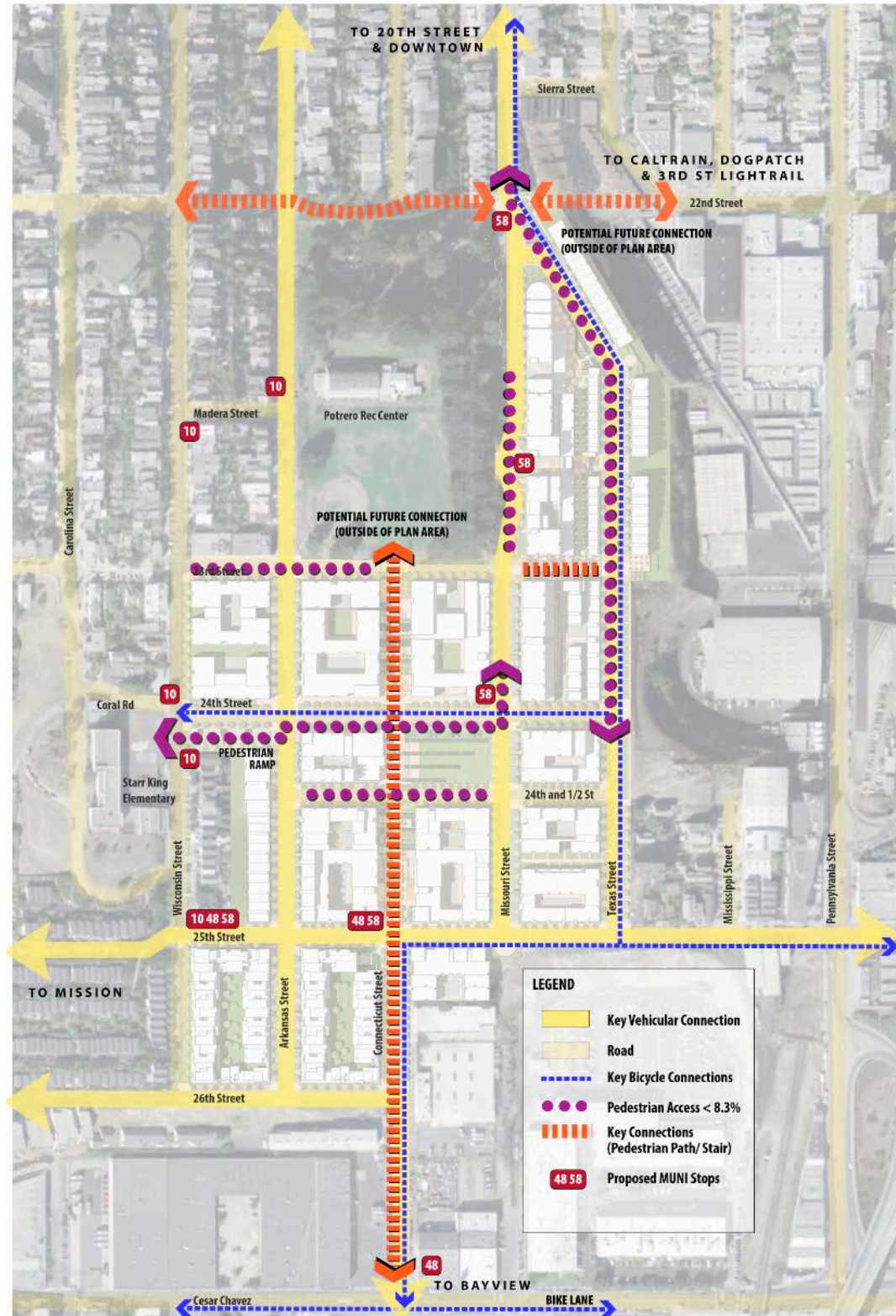
Figure 3 Planned Multimodal Infrastructure and Connections
