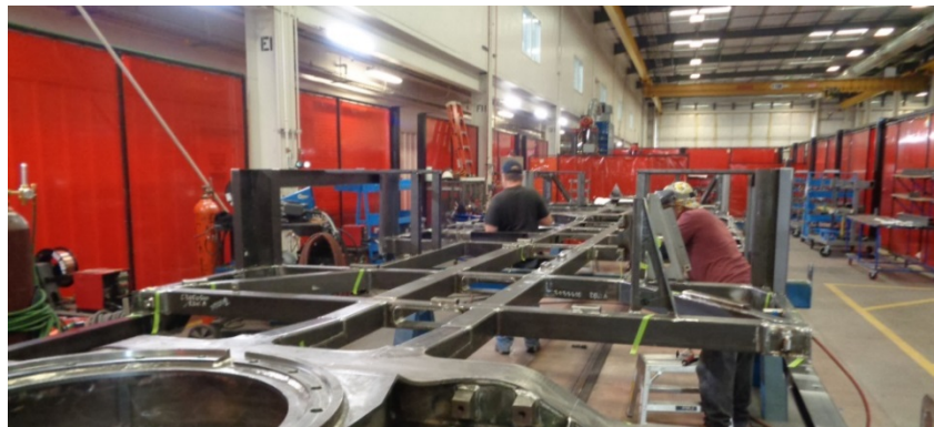
Car 4 - Underframe being welded
