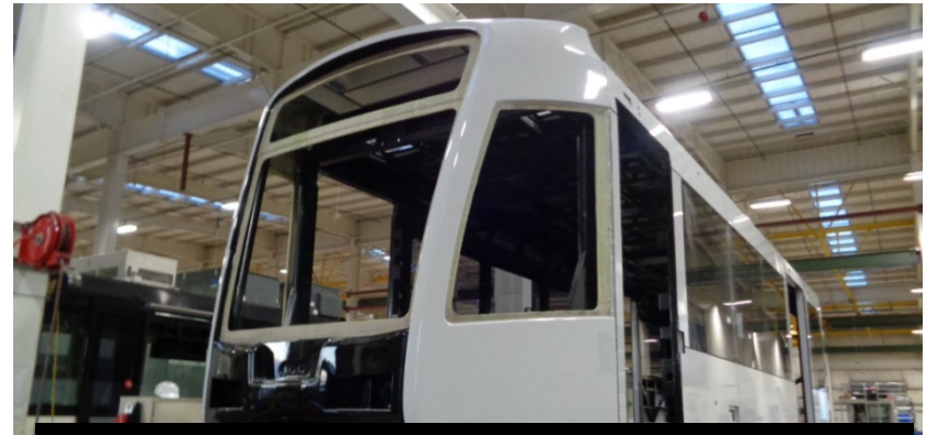
Car 2 - Car ready for floor installation
