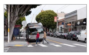
Bus bulb in Marina District: Bus bulbs were installed at stops on Chestnut Street to help riders get on and off the bus more quickly, easily and safely.
