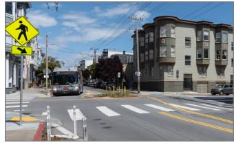
New transit-friendly traffic circle: A traffic circle replaced a fourway stop sign at McAllister and Lyon streets. Cross traffic must still stop and buses, traffic and bikes on McAllister have right-of-way.
