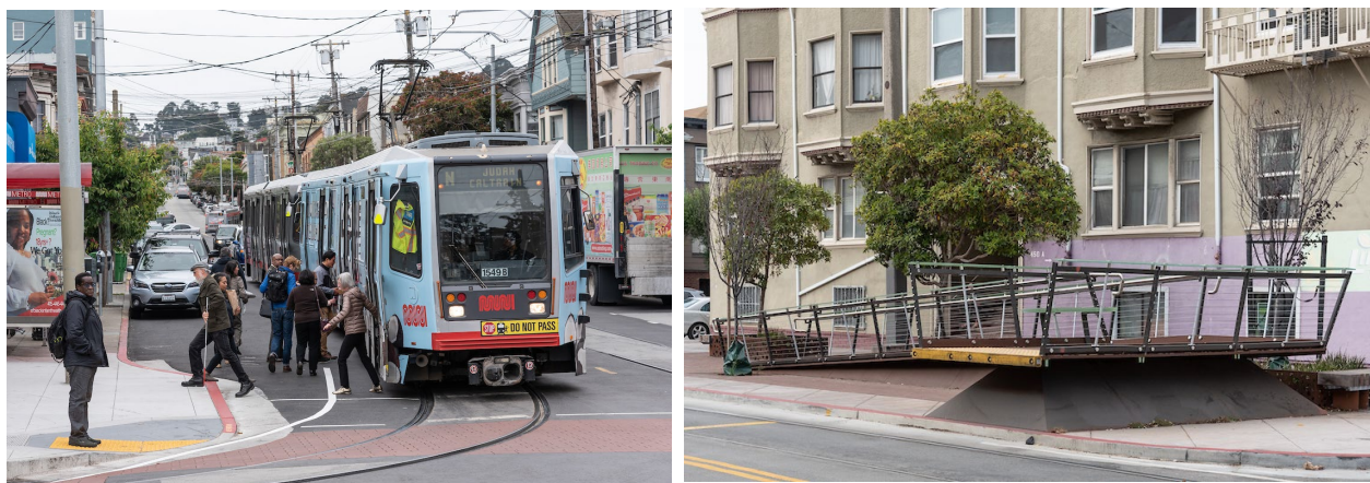
Figure 3 - Example of boarding at an inaccessible stop (left) and accessible boarding via a small ramp (“mini-high), right.
