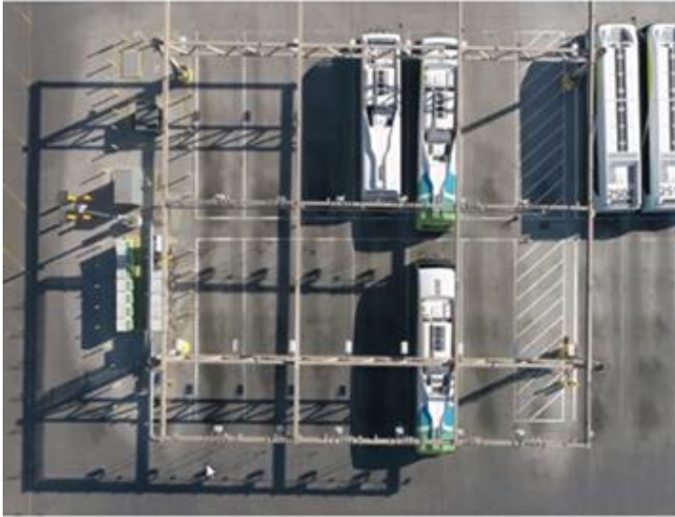
Images of Steel-Framed Gantry Structure supporting depot pantograph charging system
