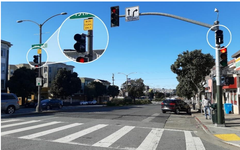
Figure 4. Muni Head Start signal (Leading Transit Interval), at 15 th Avenue outbound. These signals give Muni a few seconds head start over general-purpose traffic and were installed at six locations within the project limits.
