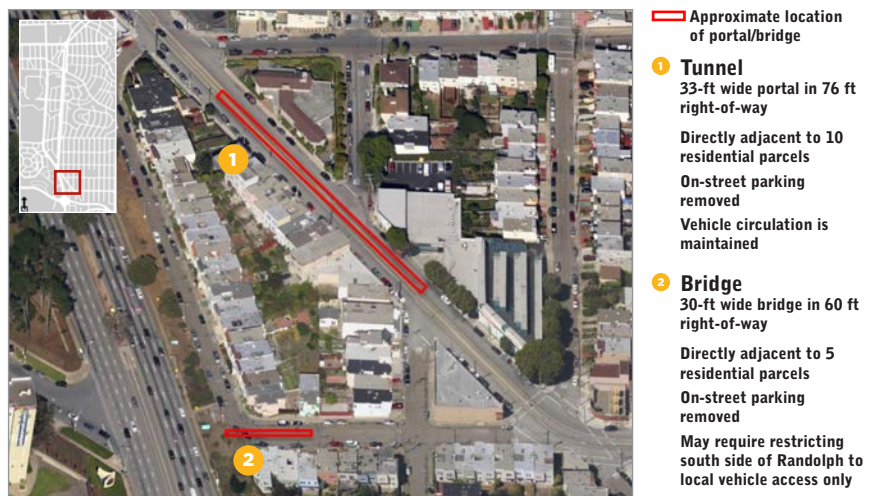
Figure 4-8. Visual, Traffic Circulation Tradeoffs: Tunnel vs. Bridge
