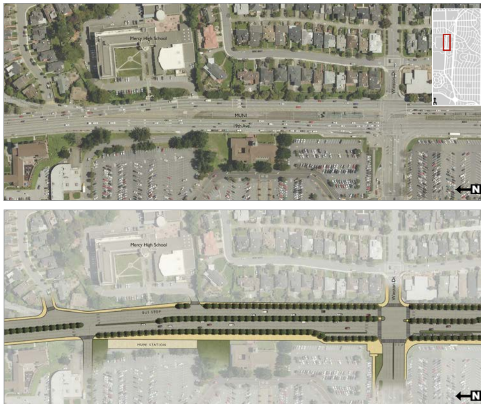
Figure 3-3. Rossmoor to Winston drives, Baseline (top), Shorter Subway (bottom), Longer Subway not pictured, similar to Shorter Subway, but southbound track remains underground on north side of Winston Drive.
