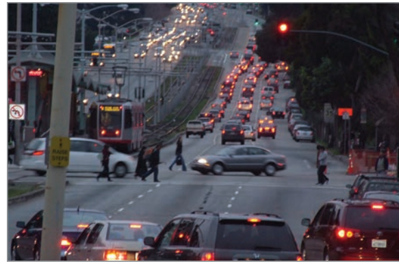
Left: The M-Ocean View must travel southbound in northbound travel lanes on 19th Avenue to enter the median near Rossmoor Drive. During peak hours, traffic often queues onto the light-rail tracks, delaying the light-rail from proceeding. Right: Access to M-Ocean View stations along 19th Avenue is challenging. Pedestrians and transit riders must cross three travel lanes to access the median stations, while avoiding conflicts with turning cars.
