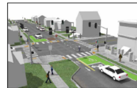
Rendering of a partial diverter at a neighborhood intersection. NOTE: see Diverter Details Board for further information.
