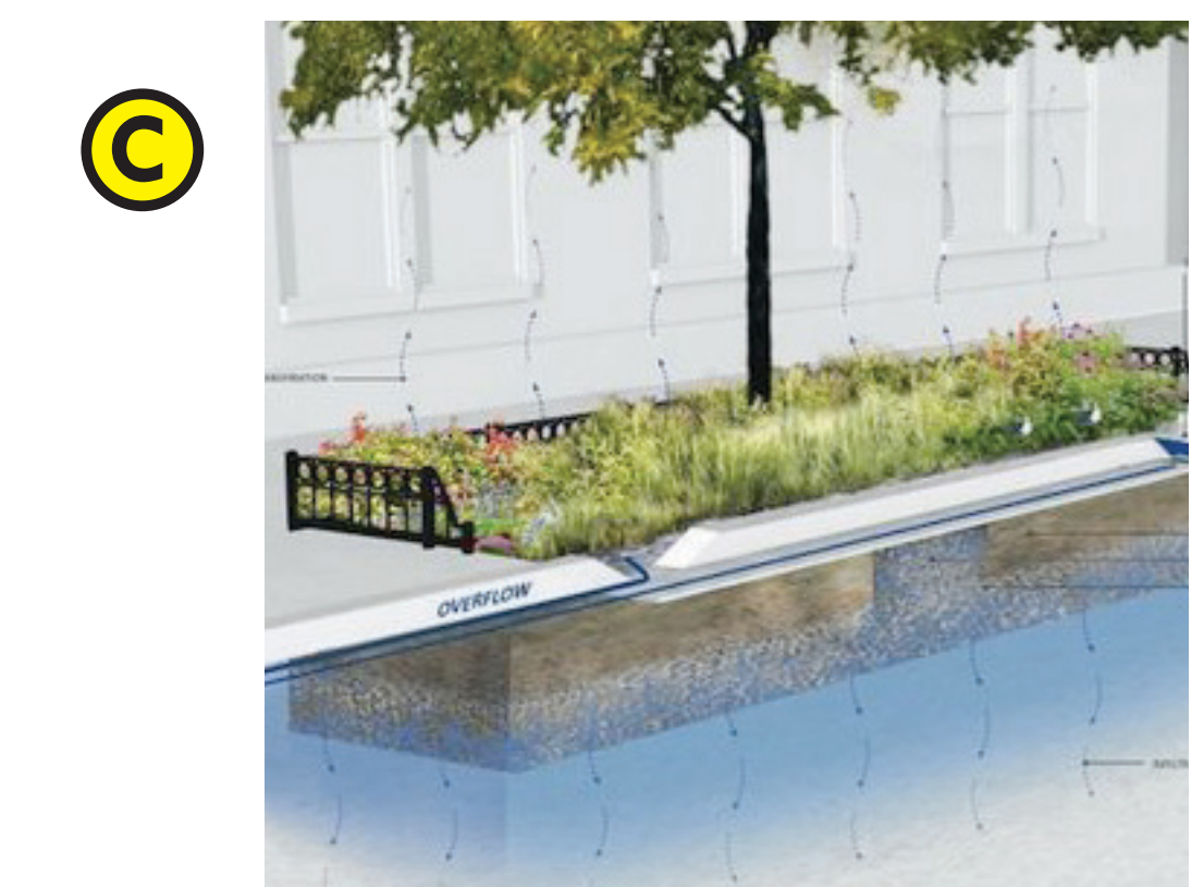
C INFILTRATION Curb openings divert street runoff into raingarden trench for stormwater infiltration
