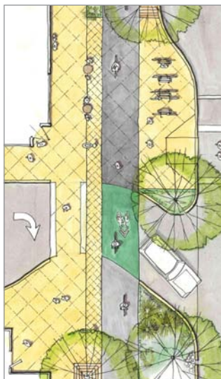
Figure 27. Integration of mid-block crossing, bulb-out, and cycletrack.
