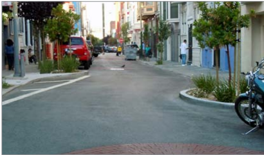
Figure 15. Chicane created by alternating on-street parking.
