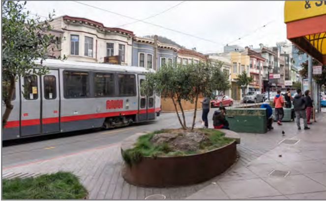
Transit bulb with landscaping (example 1 of 2): This transit bulb on 9th Avenue in the Inner Sunset is an example of transit priority and safety measures that also enhance the streetscape.
