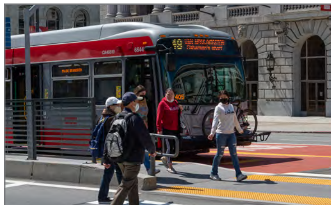
Center boarding island platforms: Passengers get on and off the bus by walking to a transit island. These boarding islands enable the bus to operate in center-running transit lanes.
