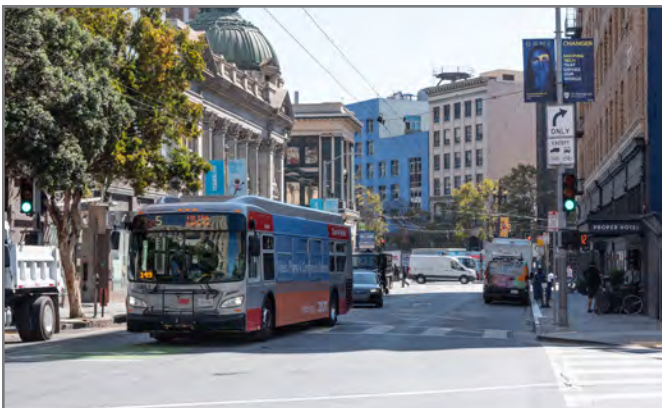
Contraflow transit lane on McAllister Street: A contraflow transit lane enabled the removal of a time-consuming "jog" in the 5 Fulton route, saving about 3 minutes per trip.
