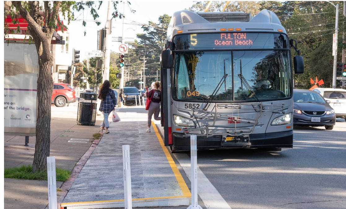
Temporary bus bulb on Fulton Street that will be replaced with a permanent concrete bulb
