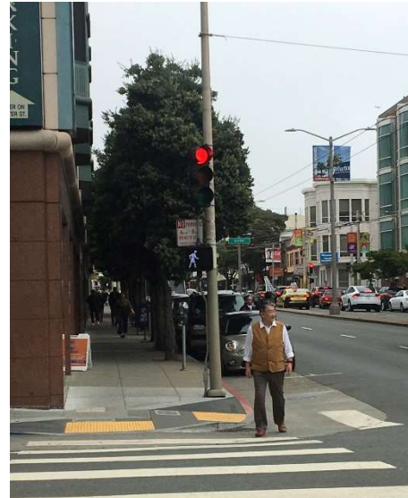
Figure 7 Example of Pedestrian Head Start Signal
