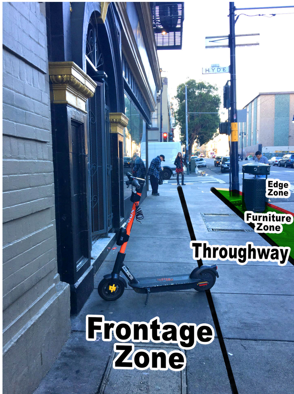
Figure 4 – Building Façade Illustration - Note how the parked Mobility Device is parked against the building façade, which impedes the path of travel, especially for blind or low-vision pedestrians. This Mobility Device also blocks the entrance to the building by requiring people entering or exiting the building to walk or roll around the device, causing an obstruction and potential tripping hazard.
