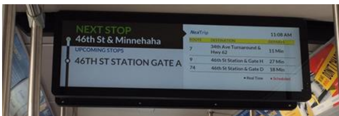
Figure 19: On-Board Digital Signage Example
