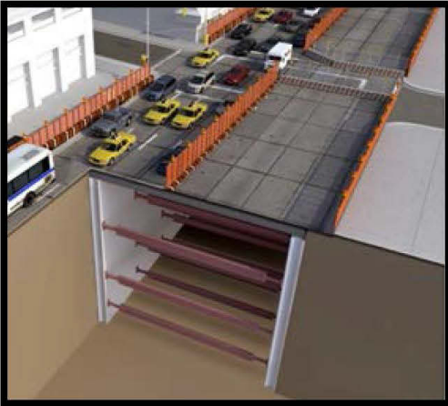
Figure 4.2.21: Typical decked street: station box construction proceeds beneath street traffic
