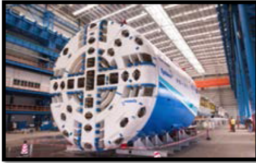
Figure 4.2.6 Pressure Face TBM “Big Alma”
